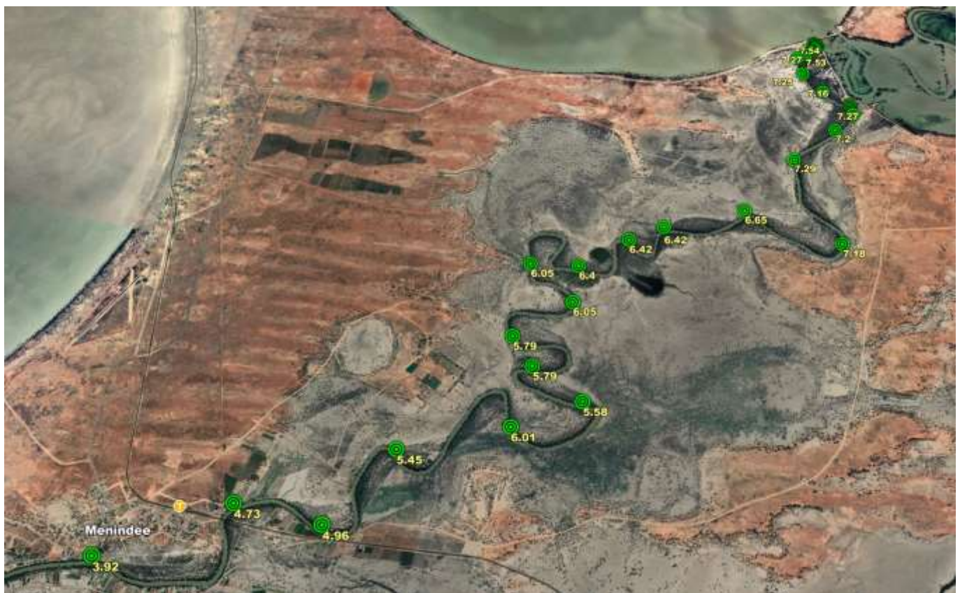
Figure 1: Google Earth image showing dissolved oxygen results (mg/L) from the Lake Pamamaroo outlet to Menindee town – 13 April
