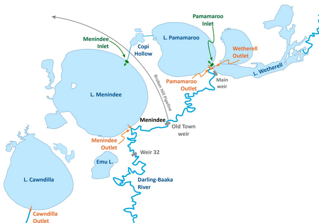
Figure 12 Menindee Lakes system. Key infrastructure regulating storage and distribution of water within the four main interconnected lakes 124
