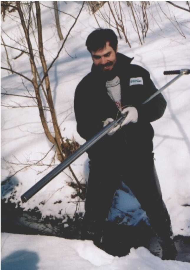
Picture 16: Sampling of sediments in surroundings of an old coal mine Jan Šverma near Lampertice at the beginning of 2004. Photo by: Jindřich Petrlík.
