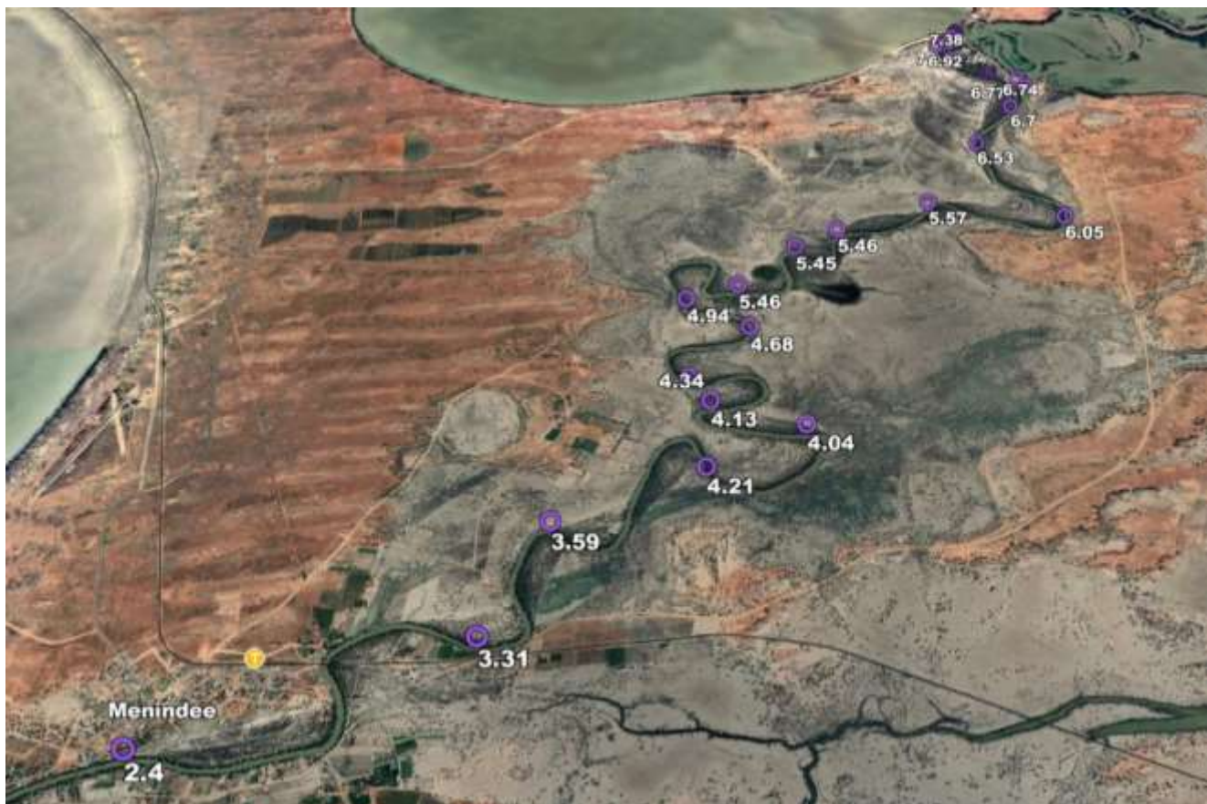
Figure 1: Google Earth image showing dissolved oxygen results (mg/L) from the Lake Pamamaroo outlet to Menindee town – 5 April
