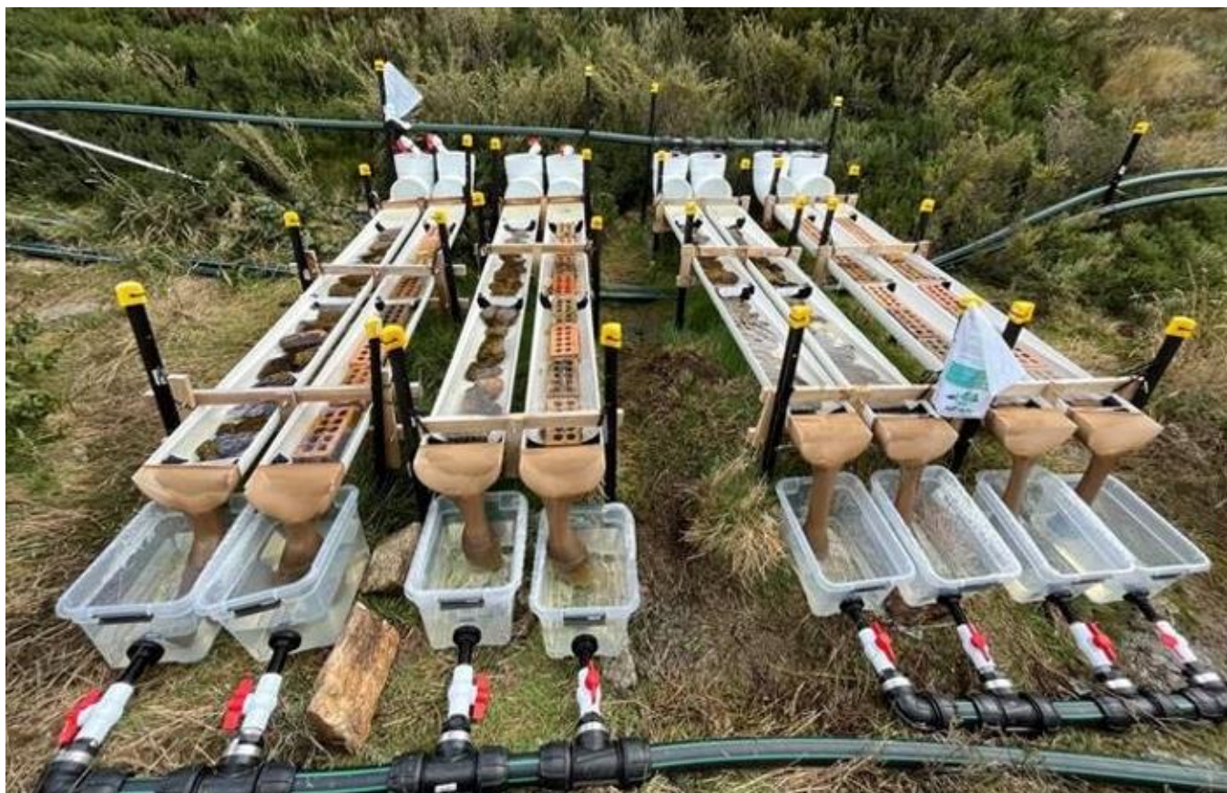
Figure 32. Stream mesocosms used in the MountainFlows component of the Australian Mountain Research Facility (Photo credit: https://www.amrf.org.au/ )
