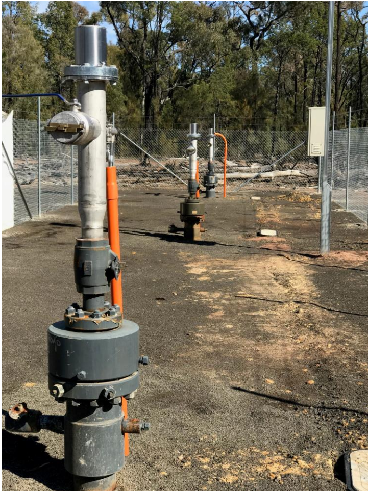
Fig 4 – Nested monitoring bores at Plumb Road (southwest of Narrabri in the Pilliga)
