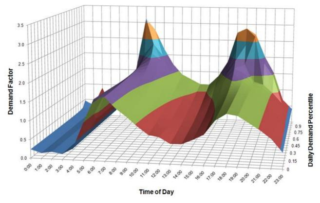
Figure 4. Example of the characterisation of a residential diurnal demand curve
