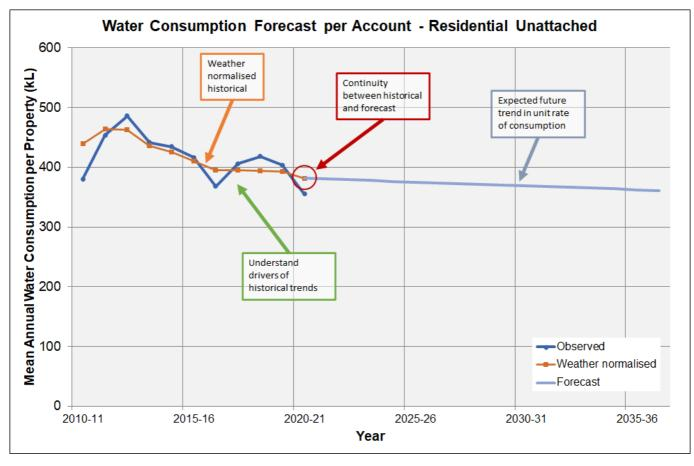
Figure 6. Analysing and forecasting unit rates of demand
