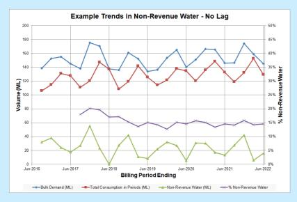
Figure 7. Assessment of trends in non-revenue water – no lag between bulk demand and customer consumption
