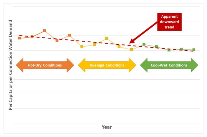
Figure 4. Weather cycles giving the appearance of a downward water demand trend
