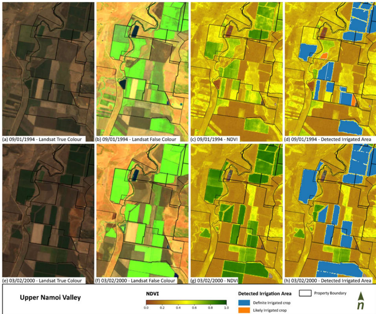
Figure 7. Examples of detected irrigation crop area for the summer cropping season in the Upper Namoi for 1993/1994 (top panel) and 1999/2000 (bottom panel). Columns from left to right: (a & e) Landsat True Colour, (b & f) Landsat False colour (Green, SWIR, NIR), (c & g) Landsat NDVI, and (d & h) detected irrigation cropping area. Landsat imagery was obtained from 'NationalMaps', Geoscience Australia.
