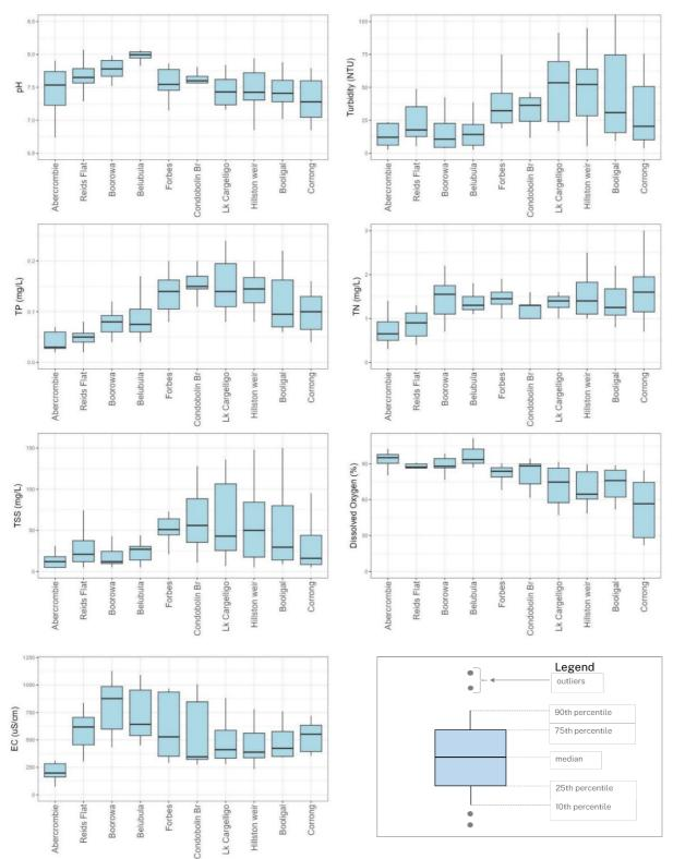
Figure 4: Water quality data by site, moving upstream to downstream from left to right. The water quality parameters shown are pH, Turbidity, Total phosphorus (TP), Total nitrogen (TN), Total suspended solids (TSS), Dissolved oxygen, and electrical conductivity (EC).
