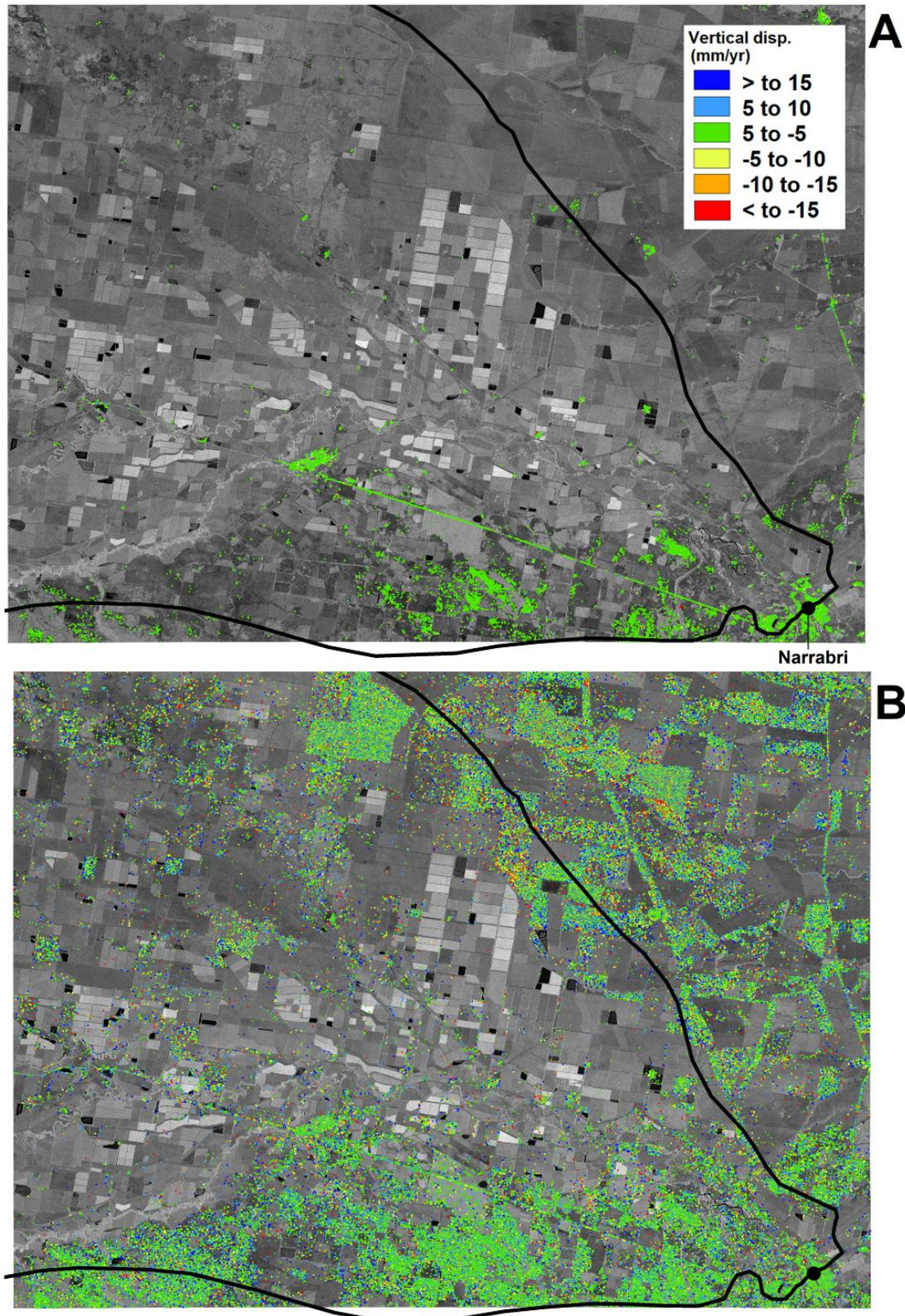
Figure 15: Results from PSI analysis over the Southwestern corner of the study area, with the groundwater flow model boundary overlaid for spatial reference. (A) Takes into account the same SAR time-series as the ISBAS-InSAR analysis, and (B) only takes into account images from 2017.
