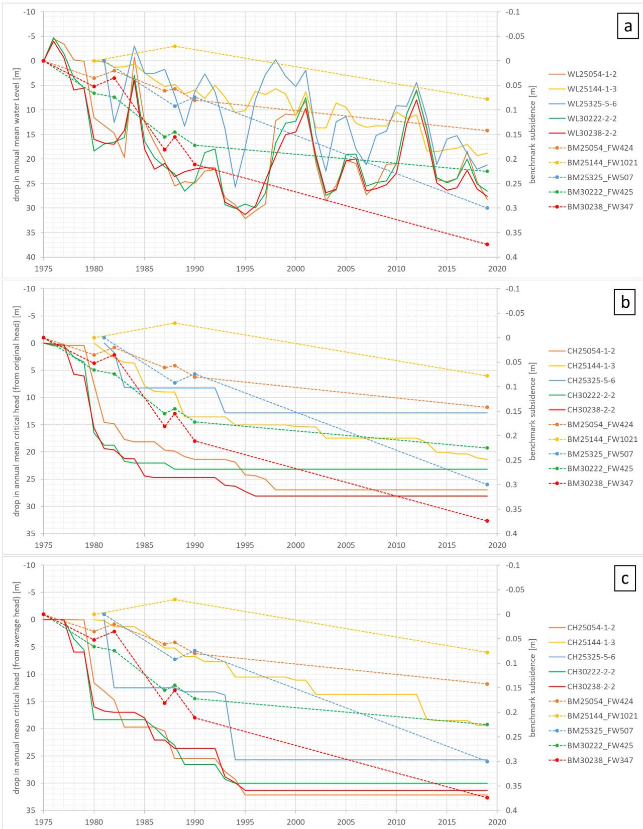
**Figure 25 Time-series of heads (WL) & critical heads (CH) with benchmark subsidence at benchmarks with >2 mm/yr (original WLS and BM subsidence (a); averaged CHs derived from original WLS with BM subsidence – Method A (b); CHs derived from average WLS with BM subsidence – Method B (c))**
