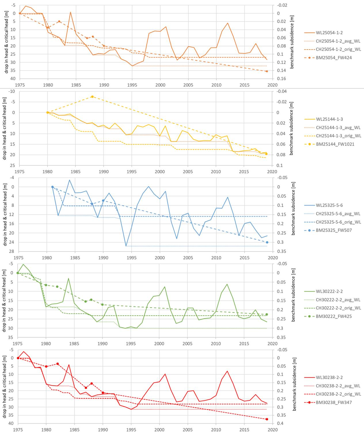
**Figure 26 Individual time-series of heads & critical heads derived by different methods and subsidence recorded at 5 benchmarks >2 mm/yr.**
