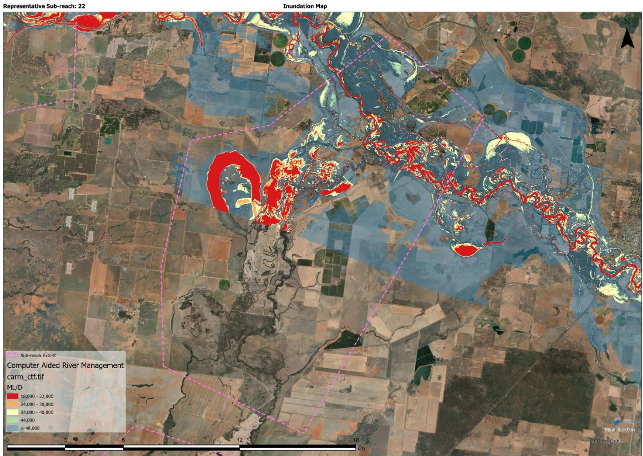
Figure 3. Inundation map for sub-reach 22.
