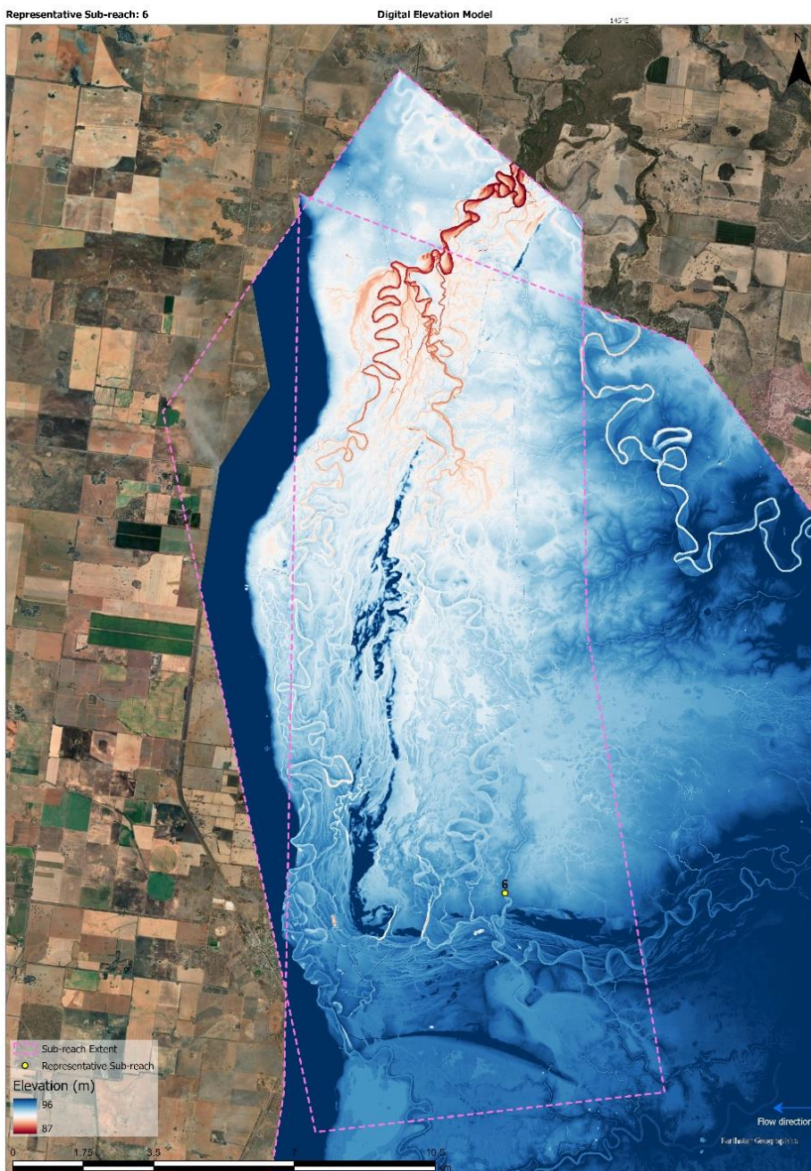
Figure 3 Lidar imagery of the sub-reach showing the different geomorphic features present
