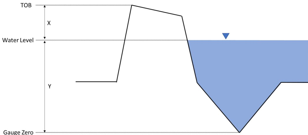
*Figure 8 Conceptual Storage Depth vs Air Space measurement*
