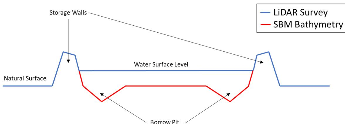
*Figure 1 Conceptual representation of an OFS and the SBM bathymetry*
