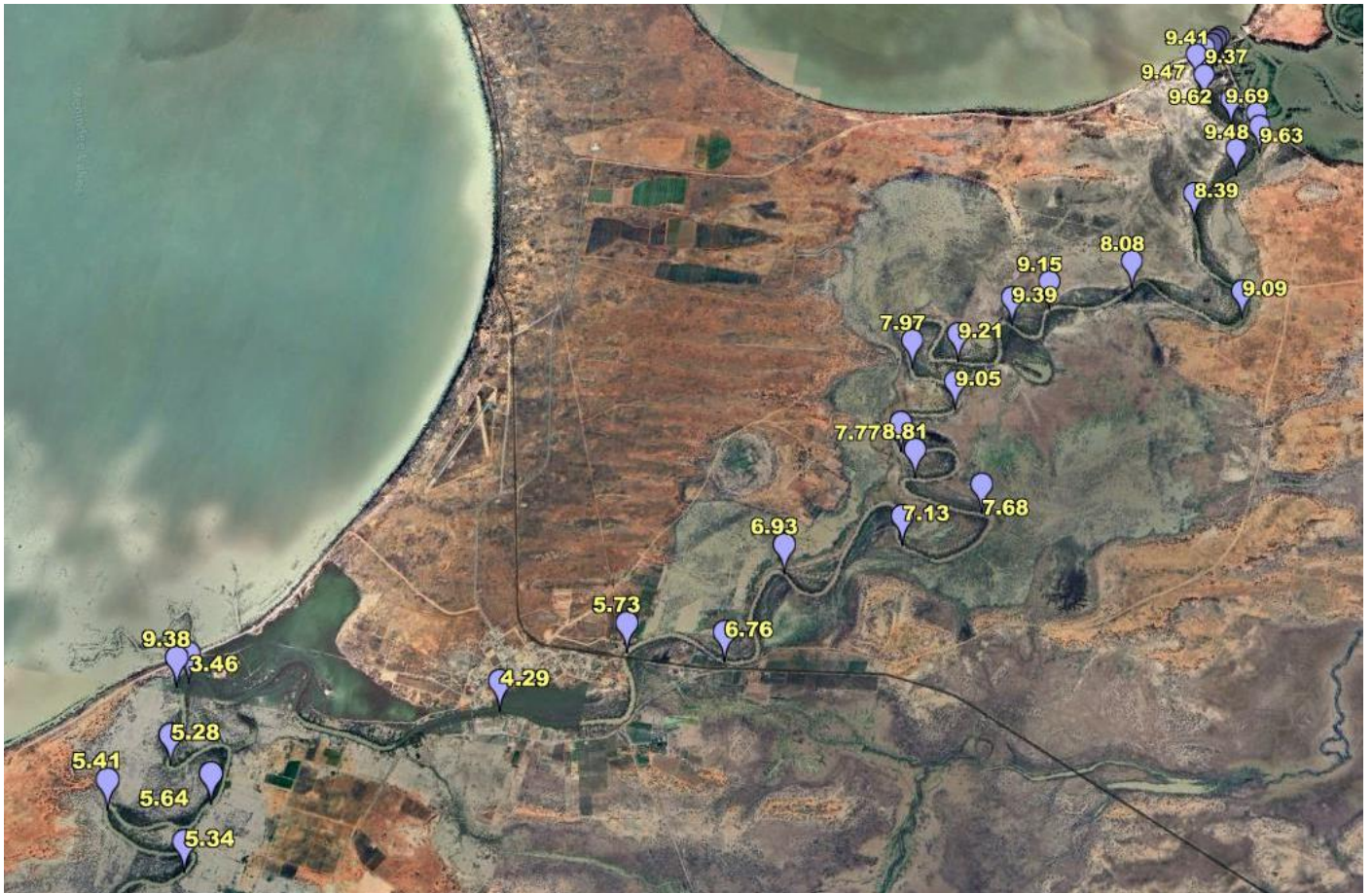
Figure 2: Google Earth image showing dissolved oxygen results (mg/L) from the Lake Pamamaroo outlet to downstream of the Darling River-Menindee Creek junction on 14 June 2023
