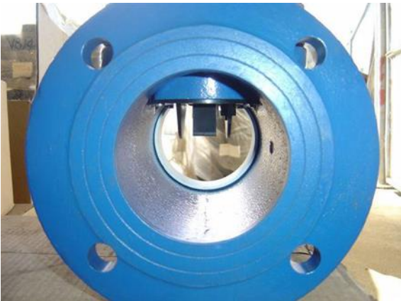
Figure 4. Example of a paddle-wheel meter
