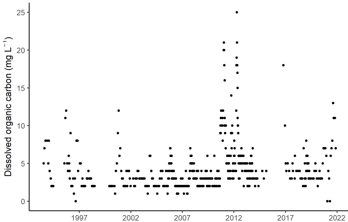
Figure 19: Observed DOC concentrations collected from Downstream Balranald Weir (410130) Data were sourced from the HYDSTRA database. Results are rounded to the nearest 1 mg.
