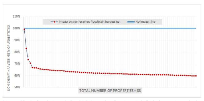
Figure 4 Distribution of change in floodplain harvesting diversions for individual properties under the Individual Impacts Scenario. The x-axis is the number of individual eligible properties represented in the Gwydir Valley model (each data point represents individual property as modelled)
