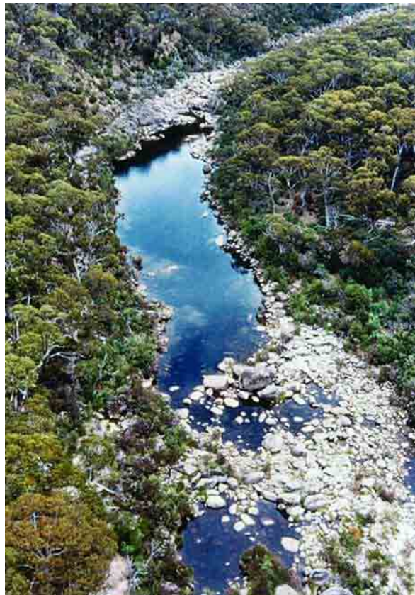
Figure 14. Snowy River below Island Bend Dam, showing remnant pool. Reconnection of these pools will be an important benefit of environmental flows. Note also the very large original channel.
