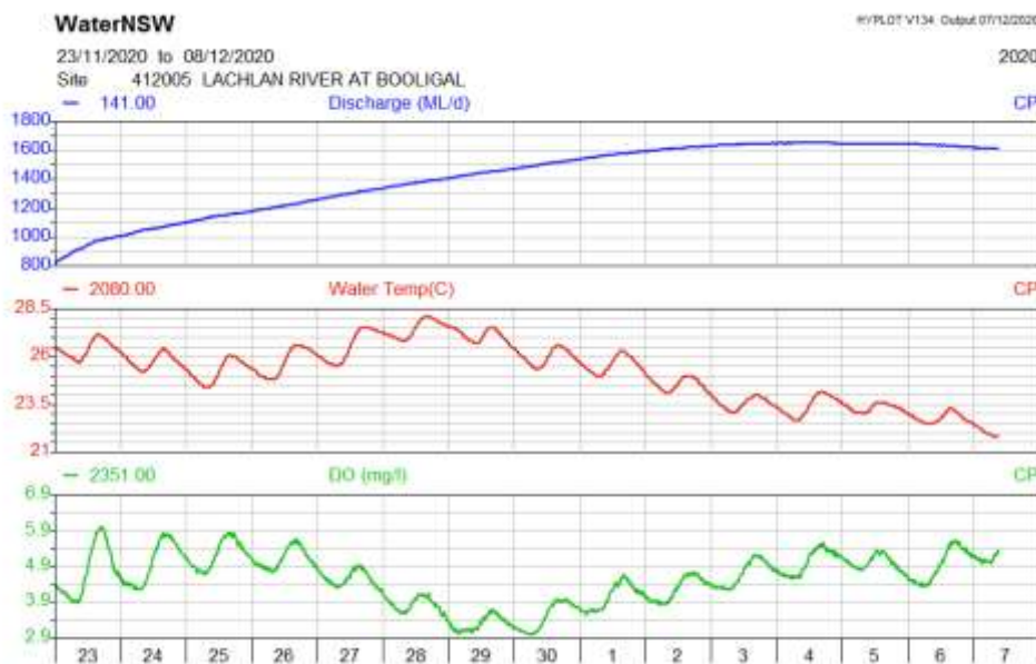
Figure 4: Discharge (ML/day), water temperature (°C) and dissolved oxygen (mg/L) in the Lachlan River at Booligal since 23 November
