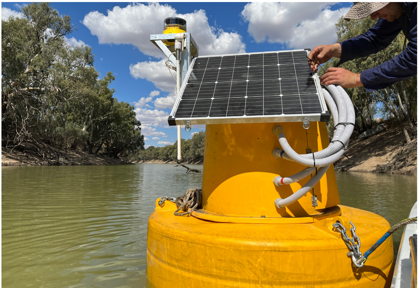
Smart-buoy measuring multi-depth water quality in real time
