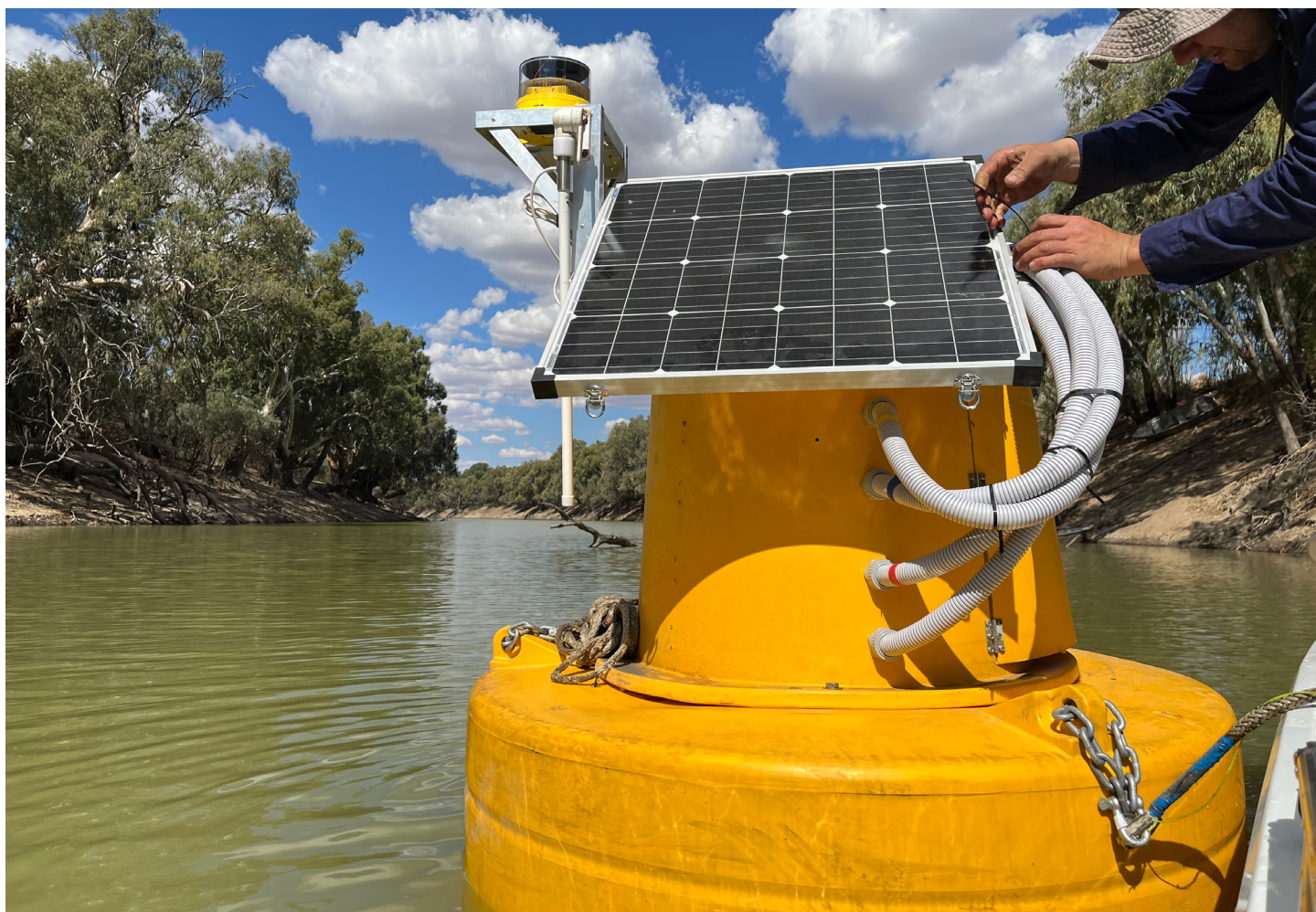
Smart-buoy measuring multi-depth water quality in real time
