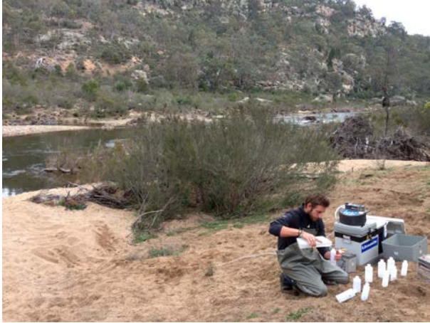
Figure 3. Sample collection from the automatic sampler unit at the Snowy River @ Burnt Hut Crossing.
